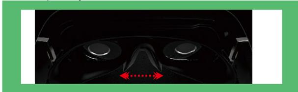
Adjust the nose pads according to the height of the nose bridge to achieve the most suitable wearing and viewing effects
